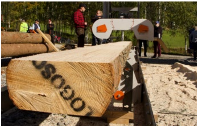
The logs are cut on two sides before you feed them into the frame saw. A unique sawing method that gives an accurate result.
