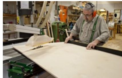
Cross cutting of board material is done quickly and safely with millimetre precision.
