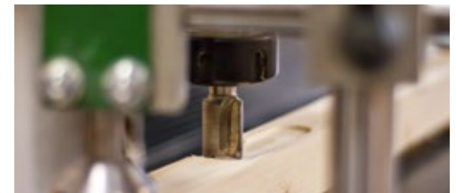
Mortising for hinges, one example of routing with the MF30.
