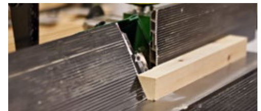
A unique feature of the MF30: tilt the rear fence to get perfect support when milling at an angle.
