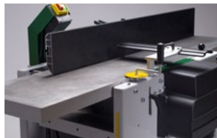
No reconfiguration! Joint on the top table, plane directly on the lower table.
