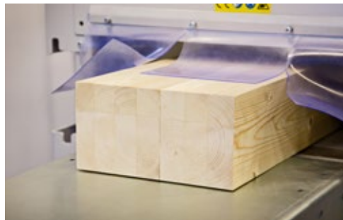
Glulam beam, machined on all four sides, with slightly rounded edges.
