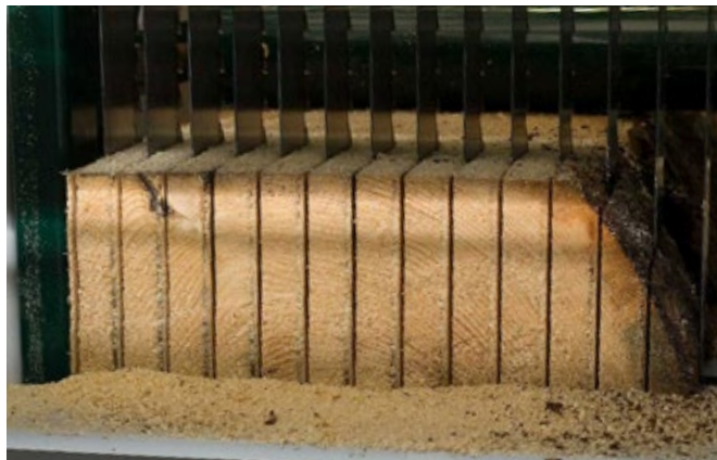
This sawing method gives an unbeatable result. The sawblades with teeth of carbide can stand up to approx. two days of full production before they need to be sharpened.
