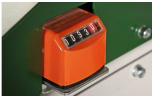
Mechanical counter for both the horizontal cutters and the side cutters.
