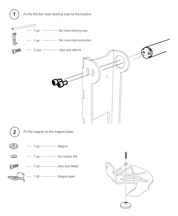
There are two different bar nose steering arms. Use the arm that is adapted for the guide bar you are going to use. Fit the magnet plate to the bar nose steering arm.
