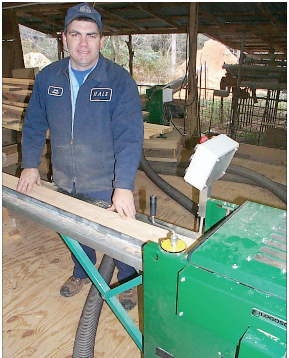
*Craig Howard with Logosol PH260 Planer-Moulder; the machine is fitted with a chip extractor also made by Logosol.*
