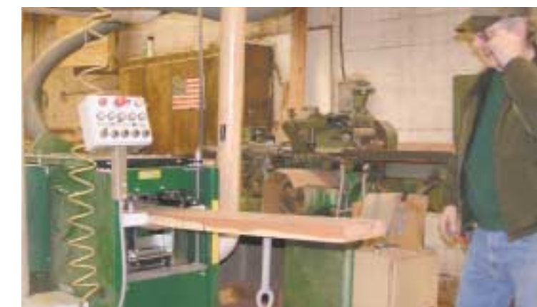
Feeding a cedar blank. It only takes one pass to convert this rough board into planed, tongue and groove closet lining. The feed rate is limited by how fast he can handle the boards.
