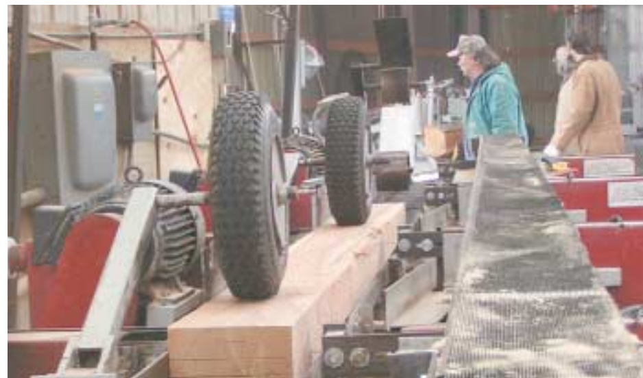
Pilot Knob has added a four-head band resaw system to their mill to saw cants into boards for cedar products, as well as oak flooring. Like the sawmill, it uses electric motors to drive the bandwheels.
