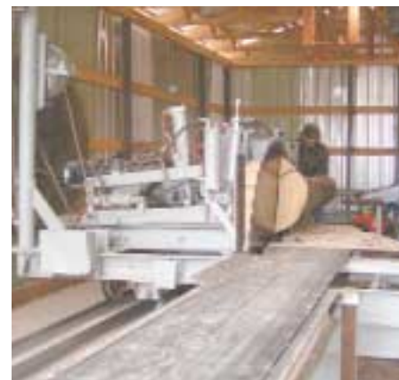
Pilot Knob Cedar Works recently replaced their bandmill with a computer controlled circular sawmill. They use the mill to cut cants, which are then sent through a resaw. They use the increased sawing capacity to cut oak flooring.
