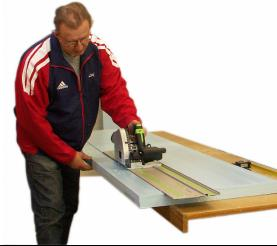
Cut the sheets to correct sizes. Straight and even cuts are necessary to make sure that the kiln will be tight.
