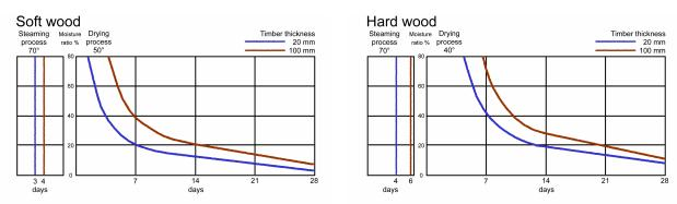
The curve chart shows the average time for the steaming process and the drying process with different assumptions. A fast increase of the ventilation will shorten the time for the drying process, but it will increase the risk for cracks.
