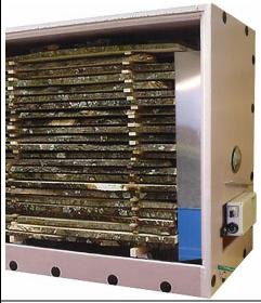
The timber is placed on bearing devices which allow the circulating air to blow under the timber. The bearing devices can be made from bricks and be connected with stiff wooden crossbars or aluprofiles. Make sure that the kiln stands on a steady bedding, because otherwise the floor of the kiln will be damaged.
