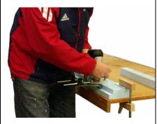
Mould rebates on roof, door, sill and sidewalls of the kiln.
