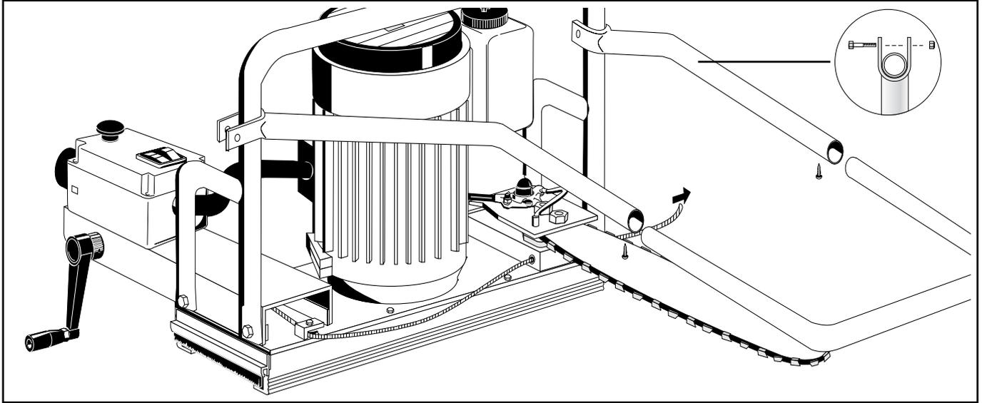
Fit the control arm to the electric saw using four M6x20 bolts and nuts. First loosen the protective yoke. Then place the control arm in position and push two bolts through the protective yoke, the control arm and its mount, tightening the nut on the inside. Use two more bolts to fasten the other side of the control arm. To tighten, use two 10 mm cap keys.
