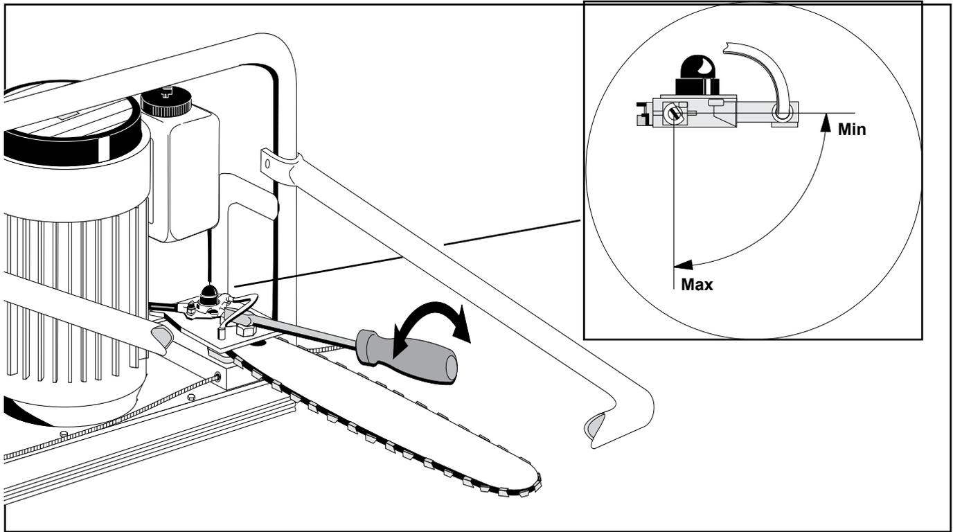
Because of the large motor effect, the oil pump is set at maximum when the chain saw is delivered. While the oil flow can be reduced, remember that there is only a quarter turn between max. and min. settings.
