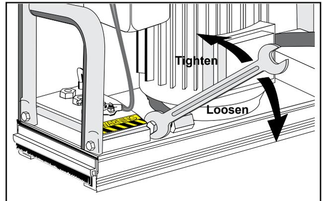
*Instructions:* Tip the saw on its side and loosen the gear bolts on the underside. Use a 6 mm hex-wrench to loosen them about one turn. Then adjust the belt tension using the setting bolt resting against the gear housing. Finish by retightening the gear bolts well.
