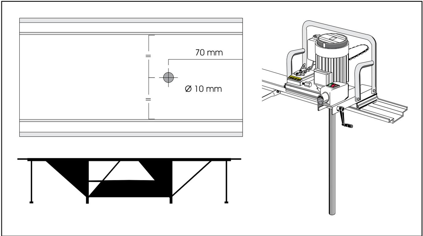
Fit the support legs to the ends of the saw mill guide rail as shown above. If the ground is loose, the saw mill and the struts ought to be attached to a wooden frame in order not to sink into the earth.
