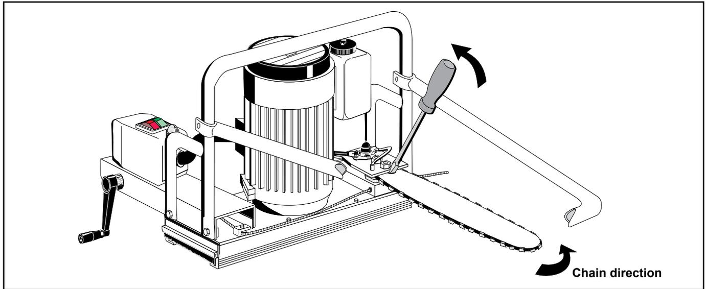
First check that the unit is unplugged. Then remove the bar nuts and the bar plate. Fit the bar and chain and return the bar plate to its place.
