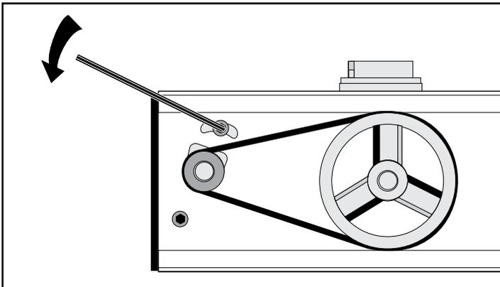
Under normal use, the Poly V-belt should last for many years. However, after some use, it may need to be tensioned in order to prevent slipping under use. For the longest working life possible, the belt should be tightened only until it engages.
