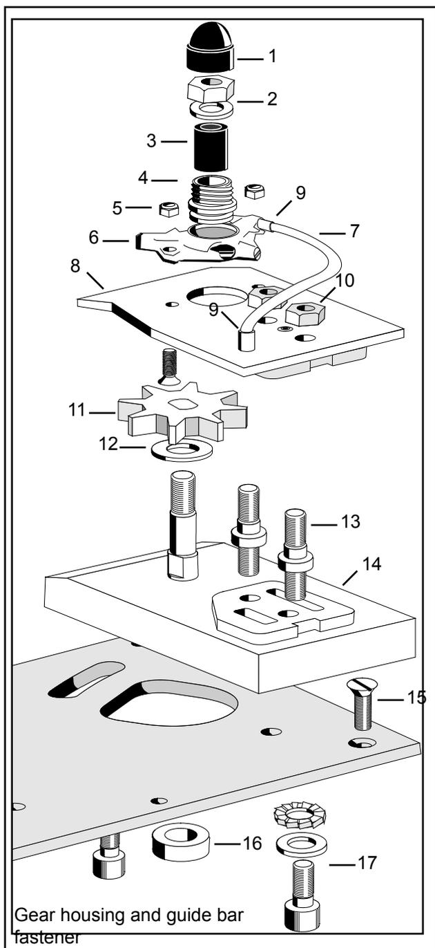
*Key Gear housing and bar fastener Art. no.*
